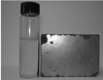
图 2 Photograph indicating the attraction of penicillin G acylase-immobilized magnetic microspheres dispersed in water by a magnet
